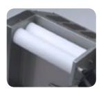
The patented balance, which does not need any adjustment, accompanies the dough from the upper to the lower rollers. The bottom dough scrapers, dough chute and plate are easily disassembled by hand for thorough cleaning.
